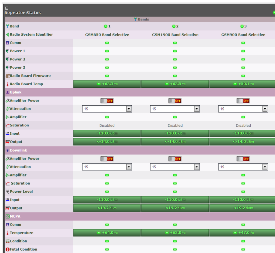
Figure 7-3: MBF-40 Repeater Status
