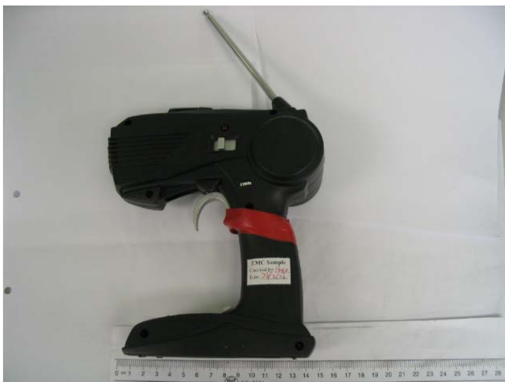
Transmitter (External view)
