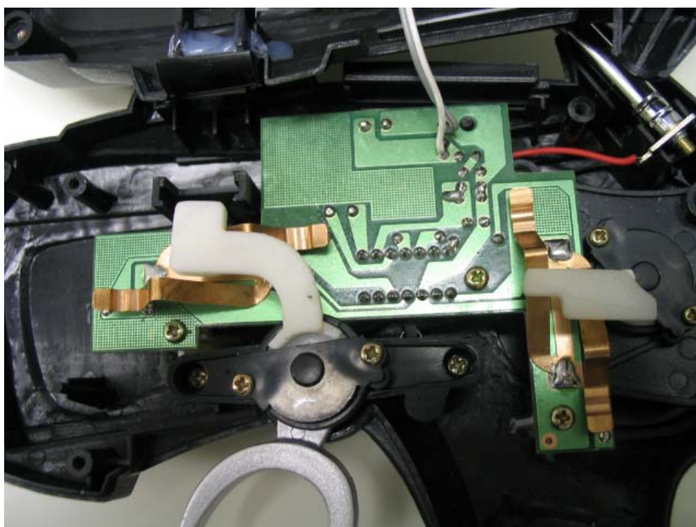
Transmitter (Internal view)
