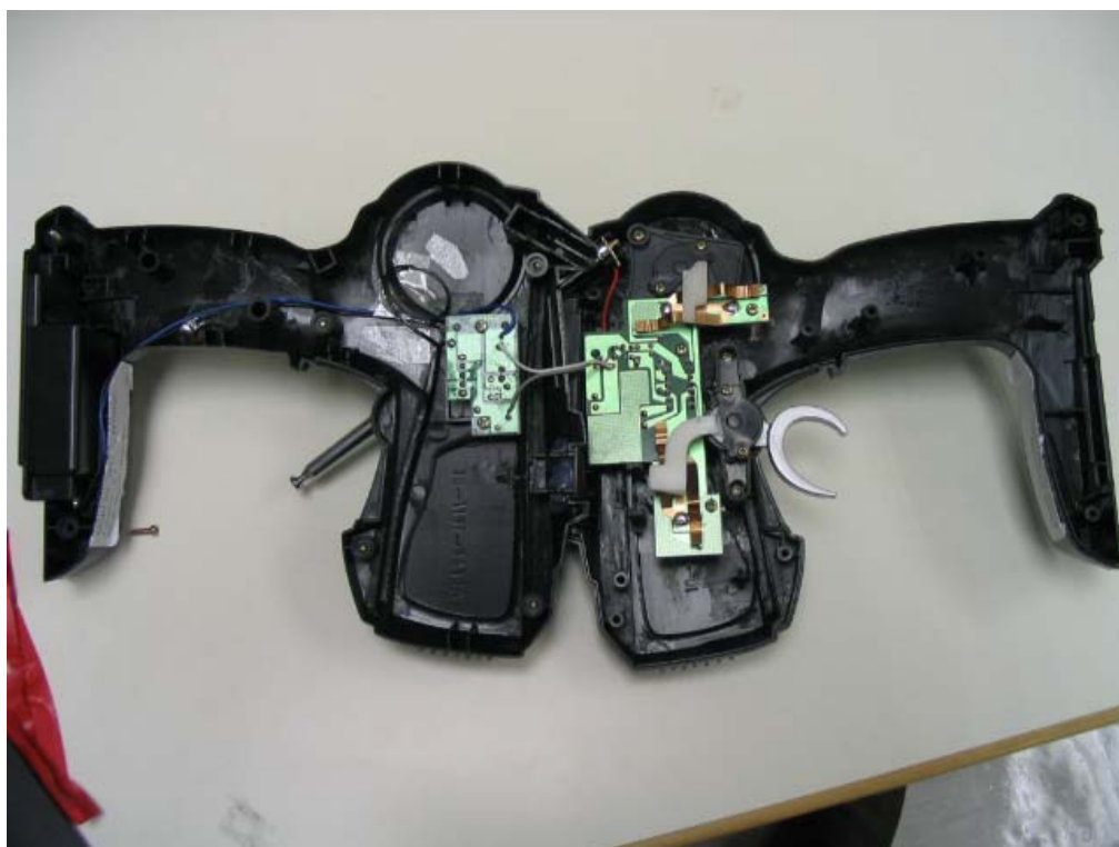
Transmitter (Internal view)
