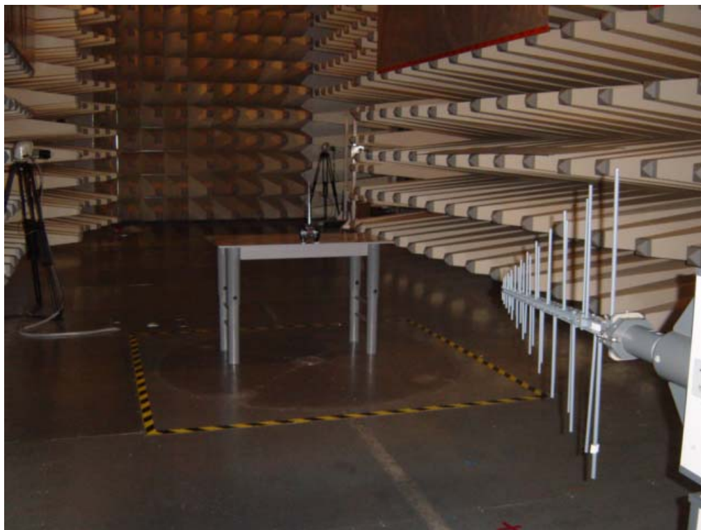
Set-up for Radiation Emission (Transmitter)
