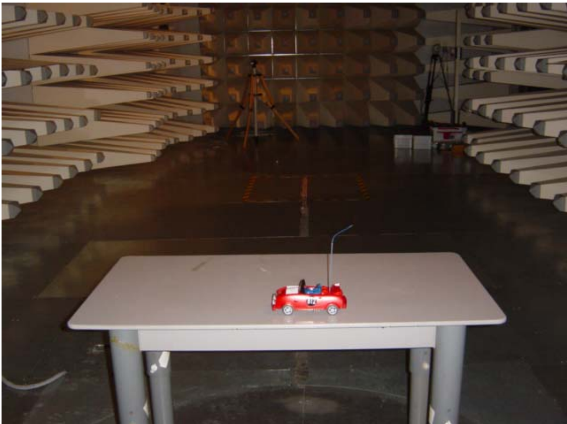
Set-up for Radiation Emission ( Receiver)
