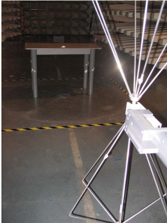
Set-up for Radiation Emission ( Receiver)
