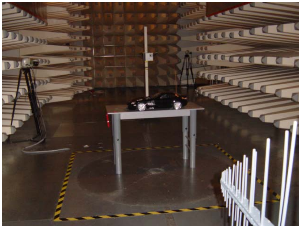
Set-up for Radiation Emission (Receiver)
