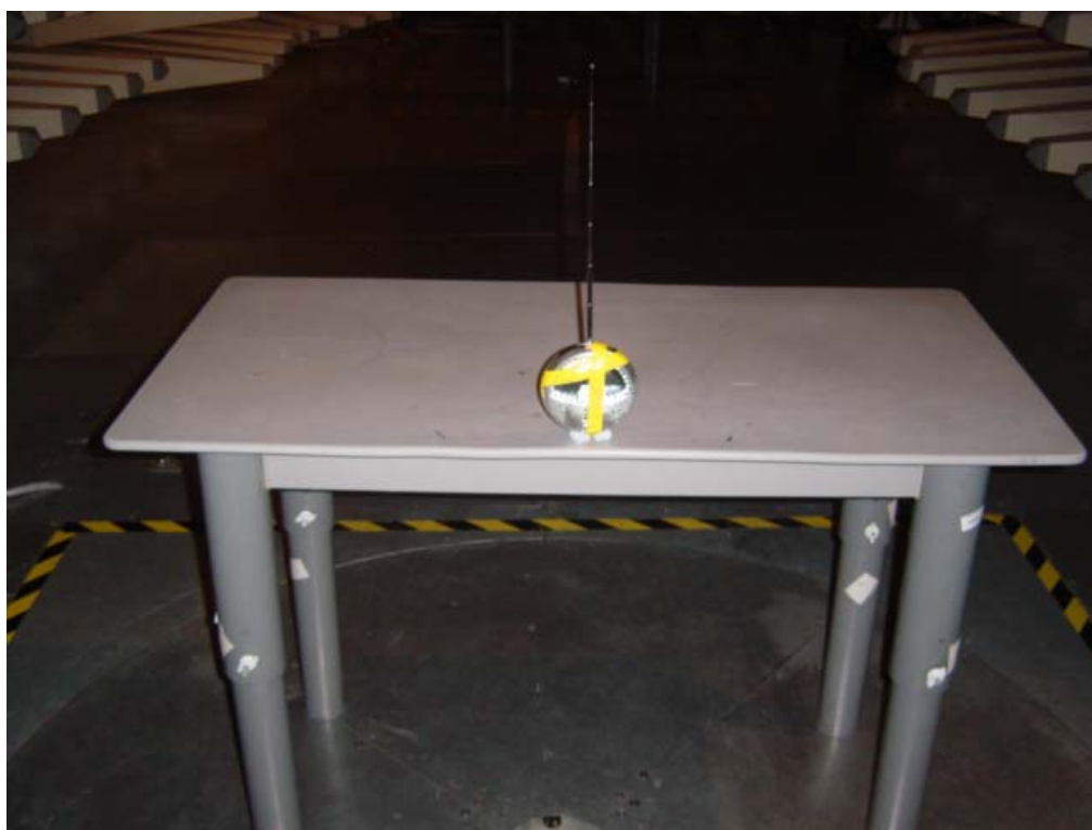
Set-up for Radiation Emission (Transmitter)
