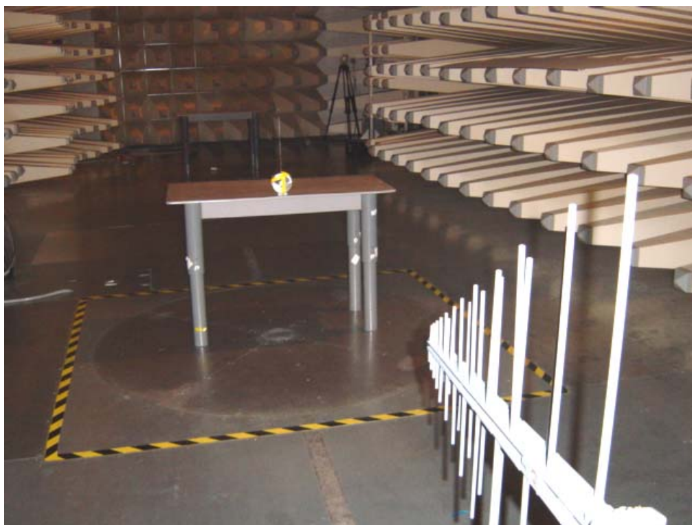
Set-up for Radiation Emission (Transmitter)
