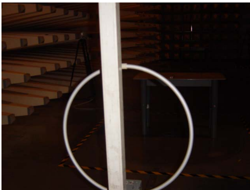
Set-up for Radiation Emission (Transmitter) using Loop Antenna
