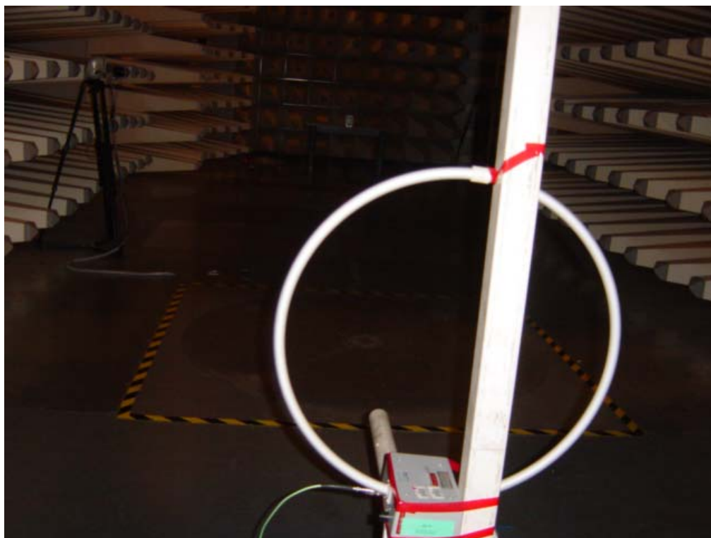
Test Setup for Radiation Emission
