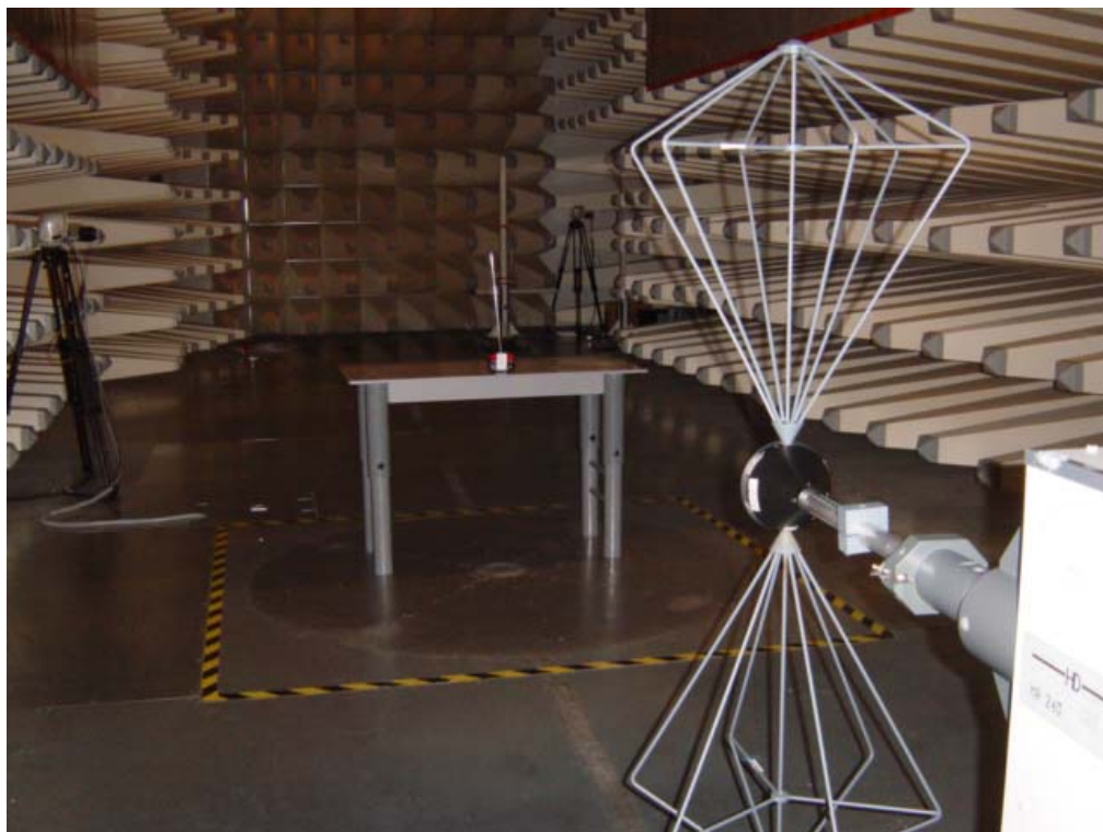
Test Setup for Radiation Emission
