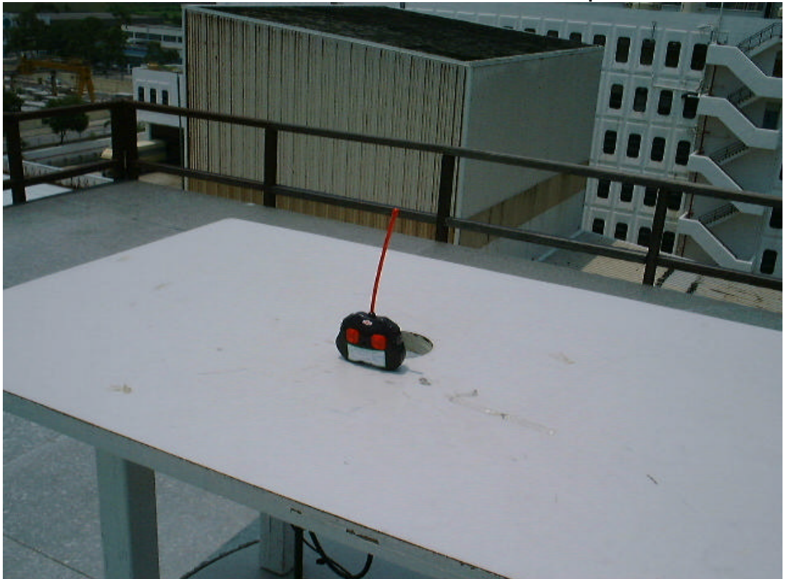
Measurement of Radiated Emission Test Set Up
