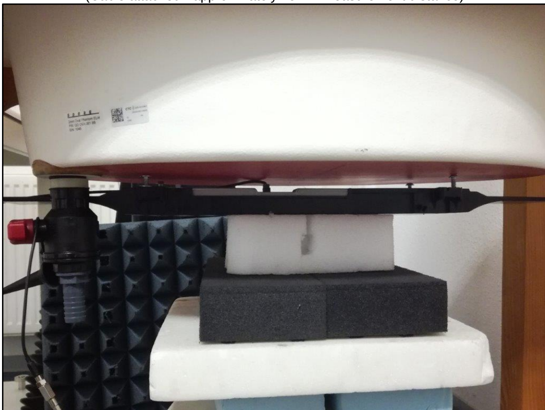
Photo 14: Test position - Antenna Type A2239059904 - Bottom side (Cable attached - approximately 15mm measurement distance)
