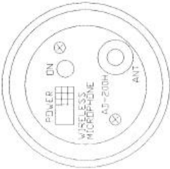
Figure 13. The bottom side panel of the transmitter.
