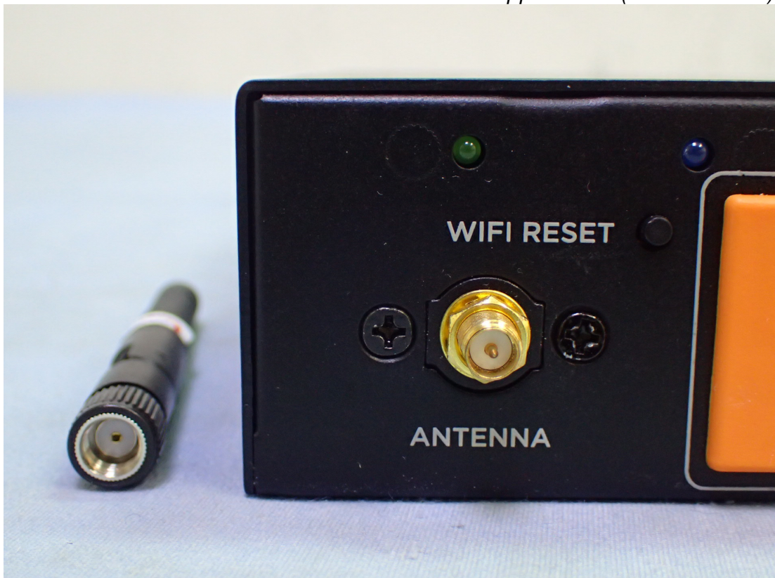
Figure 8 General Appearance (Antenna View)
