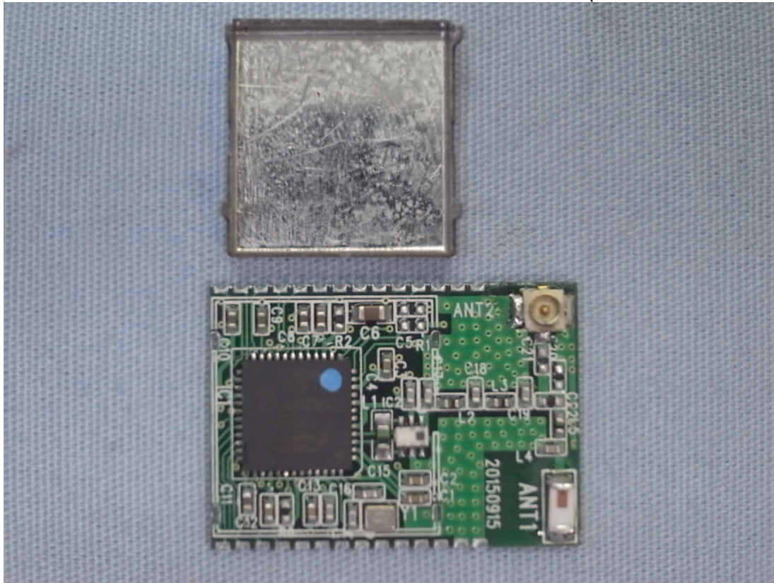
Figure 3 Internal View (Removed Shielded Cover)
