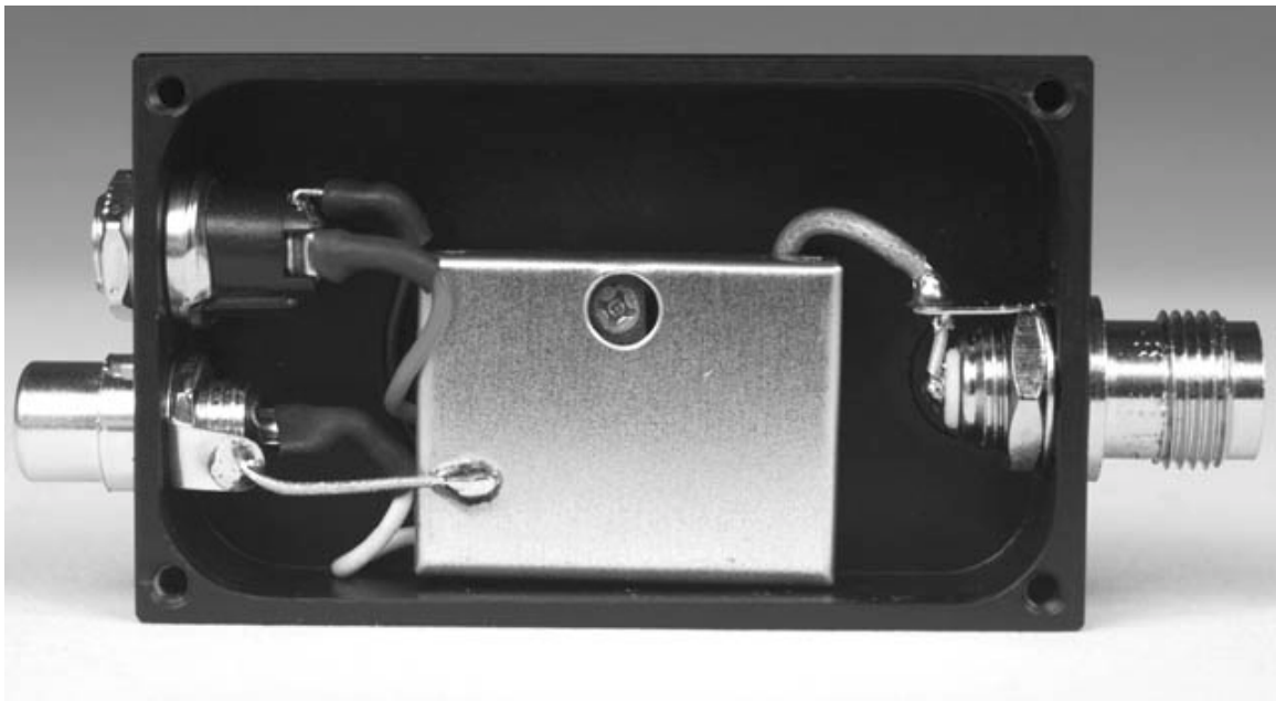
TC900 VIDEO TRANSMITTER INTERNAL VIEW
