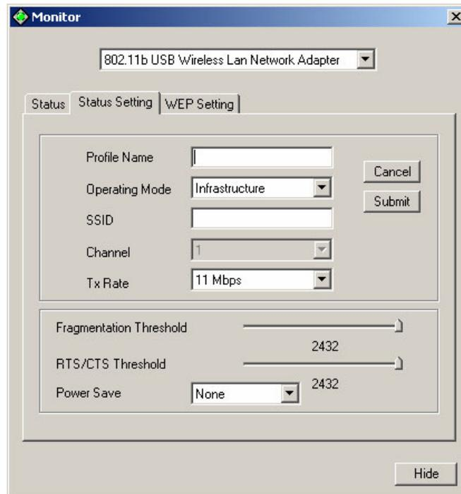
Click “**New**” in the Network page to set up the necessary parameters of the profile, and click “**Submit**” after the configuration has been changed.
