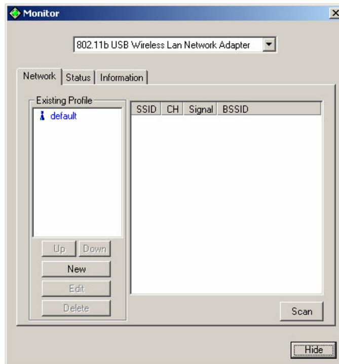
The screen at right shows all the Access Points or Adapters nearby when operating in Ad-Hoc mode. Click "**Scan**" to collect the SSID and Channel information of all the wireless devices near by.
