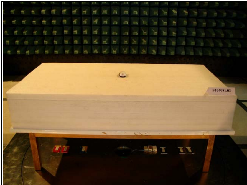
Radiated Emission Test
