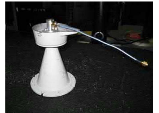
A transition is attached to each antenna.
