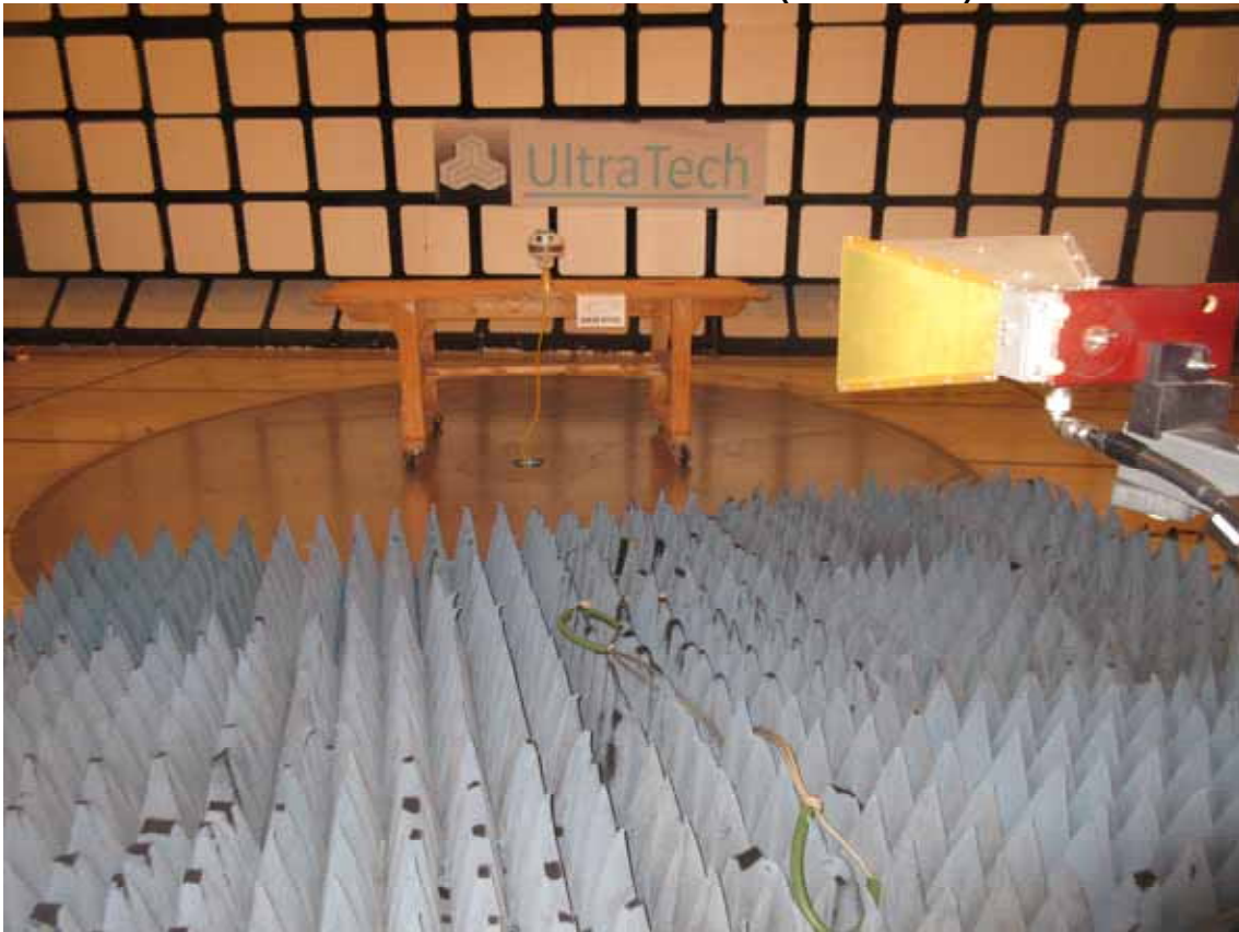
Radiated Emissions at 3 m Distance (above 1 GHz)
