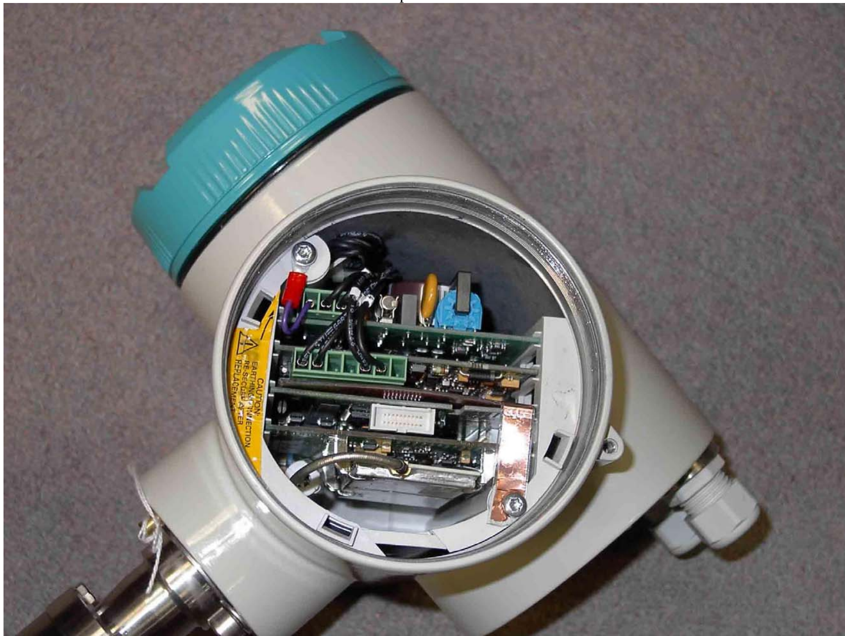
Board Stack placed into enclosure
