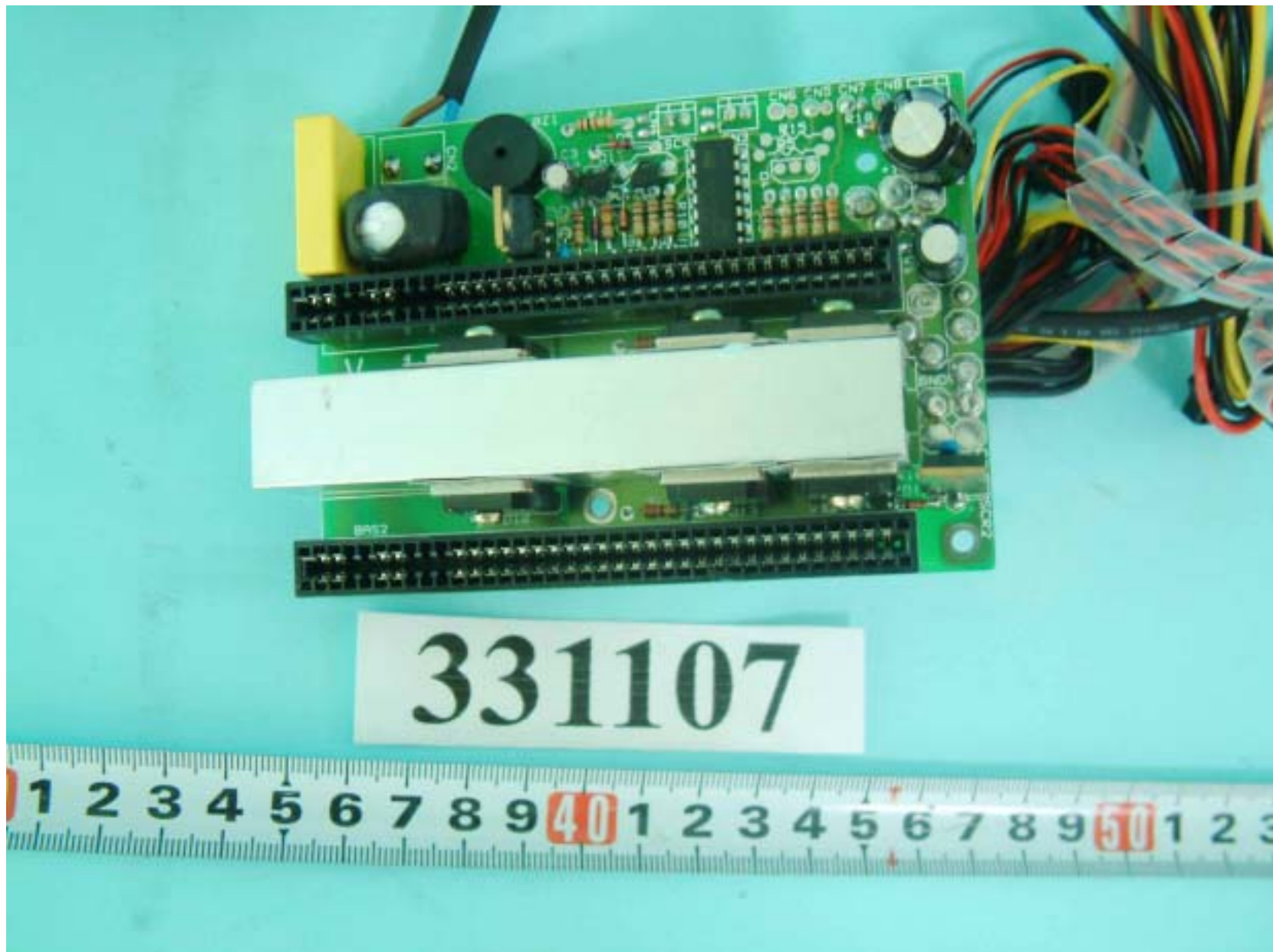
Front side of back plane of power
