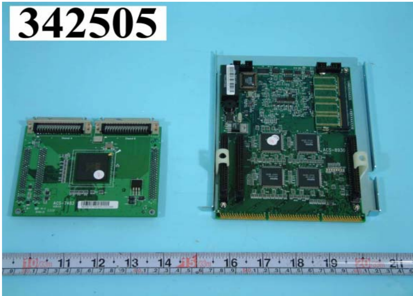
Front side of SCSI daughter board and Controller
