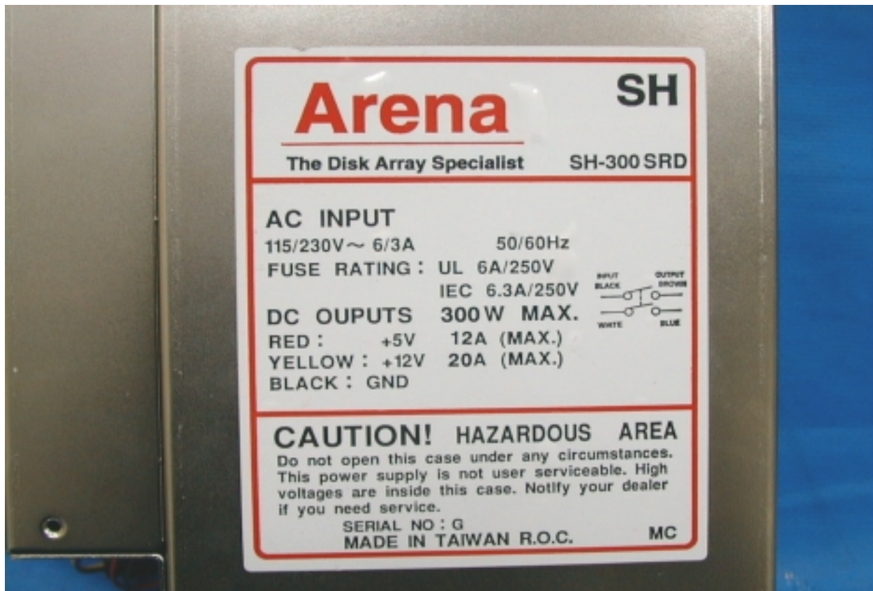
PHOTO. 15. POWER SUPPLY LABEL VIEW
