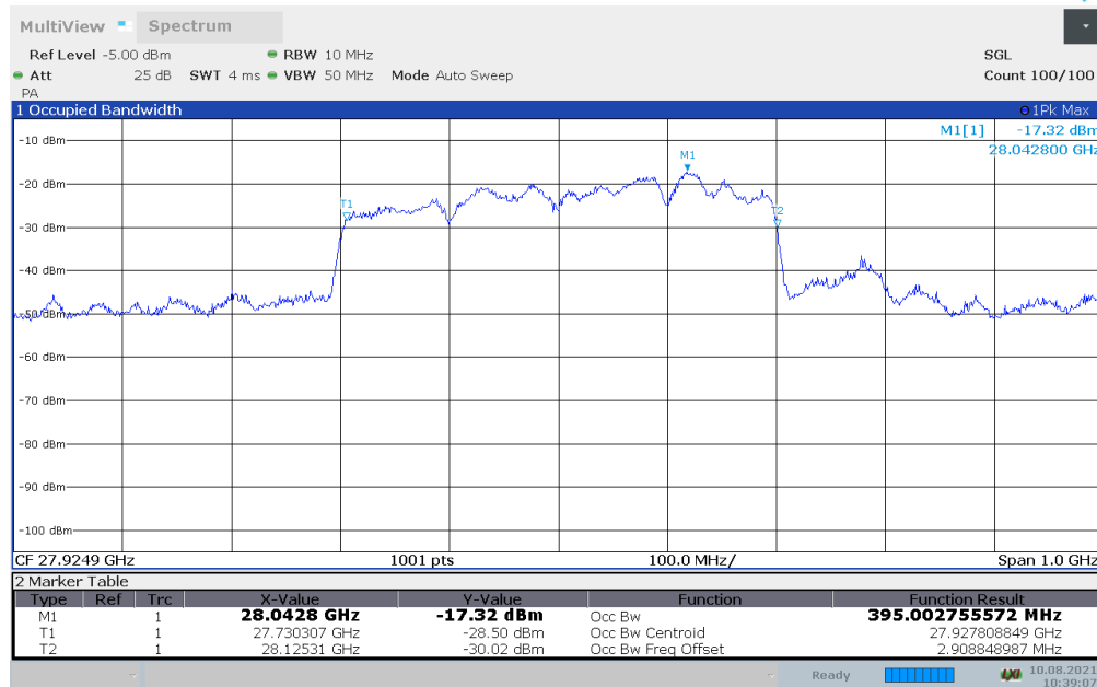
Plot 7-8. Occupied Bandwidth Plot - (n261 100MHz - 64QAM - Mid Channel) – Donor Side – H Beam
