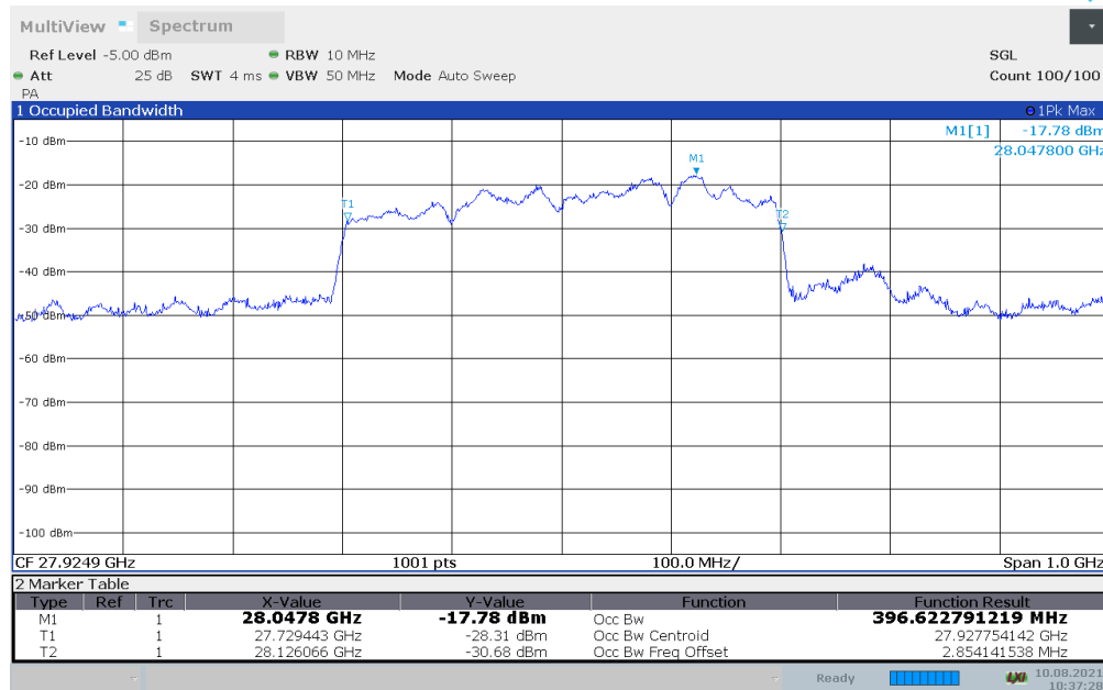
Plot 7-6. Occupied Bandwidth Plot - (n261 100MHz - QPSK - Mid Channel) – Donor Side – H Beam
