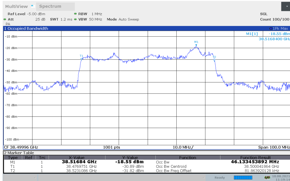
Plot 7-33. Occupied Bandwidth Plot - (n260 50MHz - \pi/2 BPSK - Mid Channel) – Donor Side – H Beam
