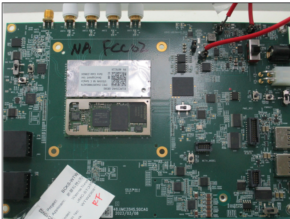
Without shielding case (only MCU, PMIC, Crystal, EMMC component)
