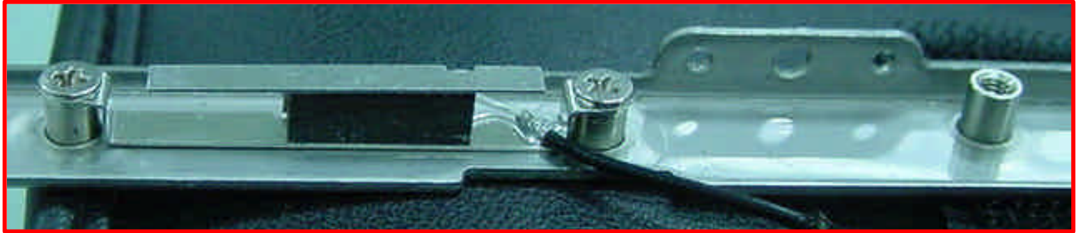
Initial antenna assembly
