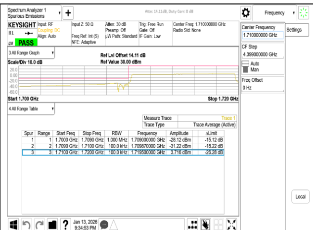
Band66 10MHz CP OFDM SCS15kHz QPSK RB52_0 CH343000
