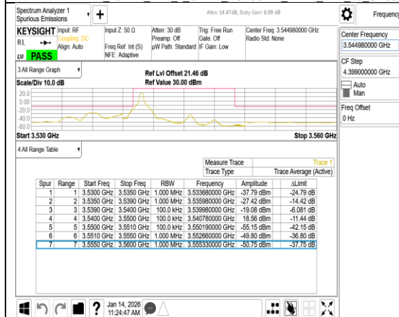
Band77-Part27 10MHz DFT s OFDM SCS30kHz BPSK RB1 0 CH636332
