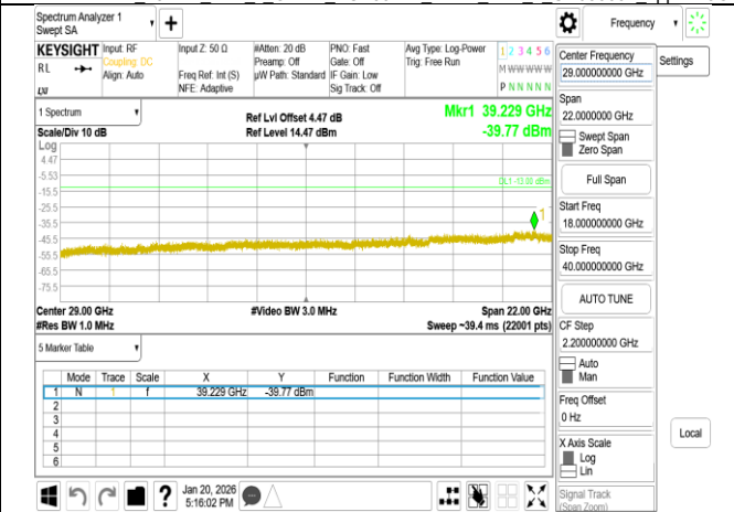
Band77-Part27 15MHz DFT s OFDM SCS30kHz BPSK RB1 1 CH636166 upper 18G
