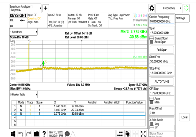
Band66 5MHz DFT s OFDM_SCS15kHz BPSK RB1 1 CH349000 below 18G
