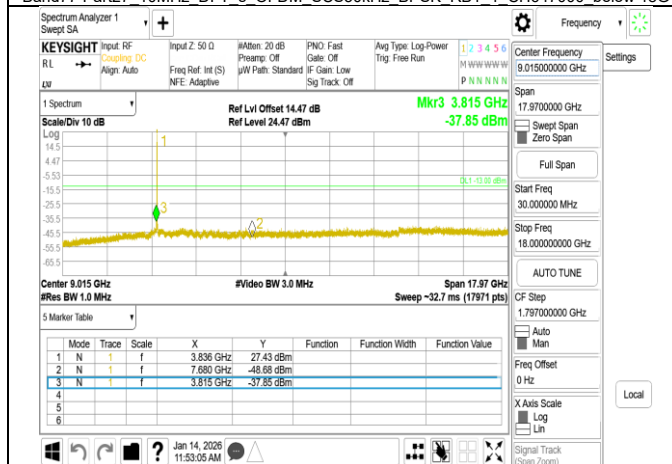
Band77-Part27 10MHz DFT s OFDM SCS30kHz BPSK RB1 1 CH656000 below 18G
