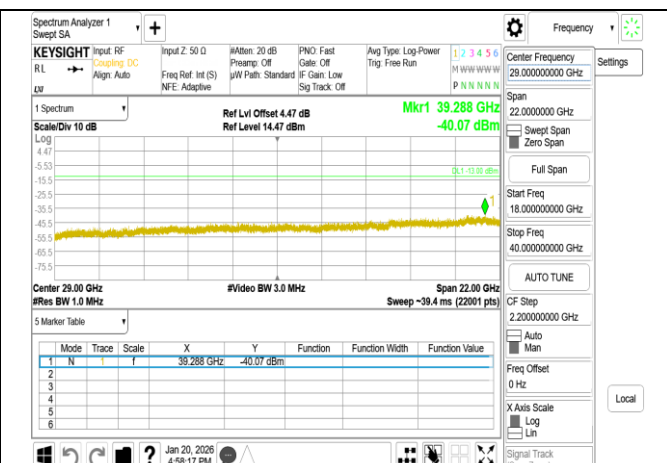
Band77-Part27 10MHz DFT s OFDM SCS30kHz BPSK RB1 1 CH647000 upper 18G
