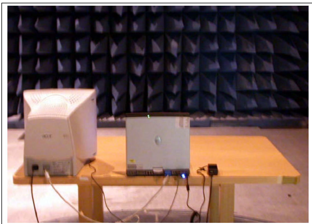
The Back View of Highest Radiated Set-up For EUT
