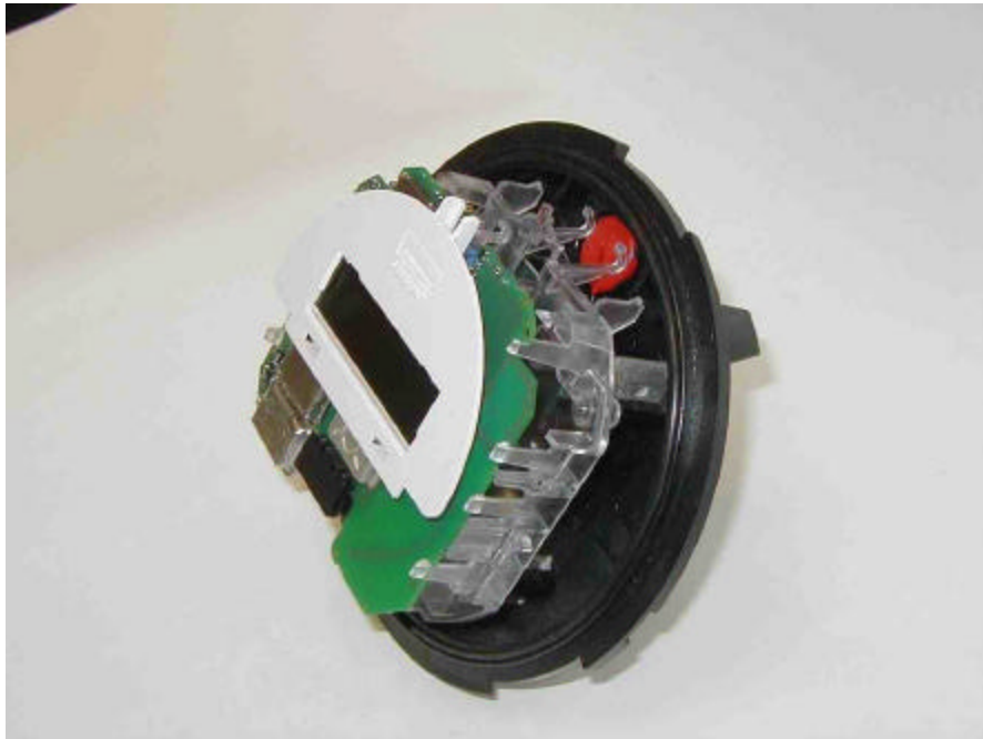
Figure 93 Printed Circuit Mounted in Housing
