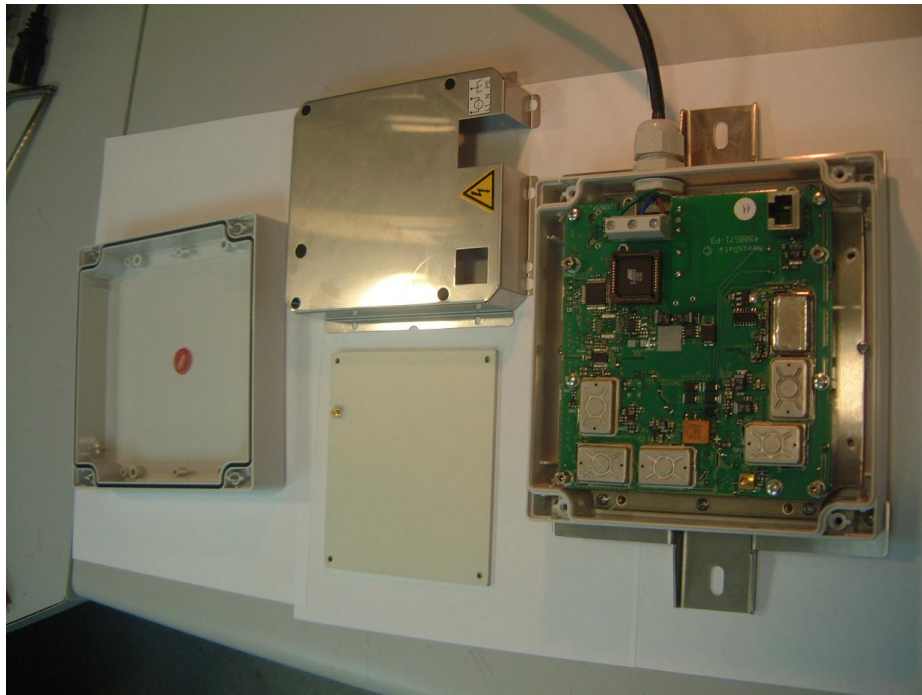
Printed Circuit Mounted in Housing/ E.U.T. Disassembled
