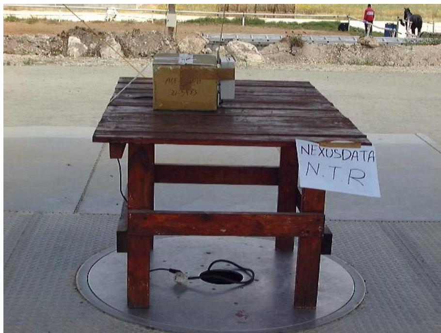
Figure 4. Radiated Emission Test. Side
