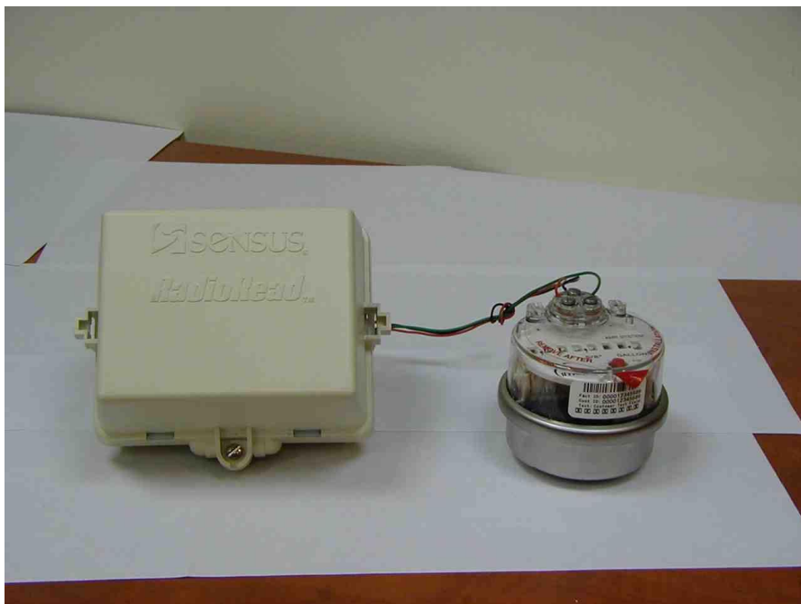
Figure 2 Transmitter Connected to Water Meter
