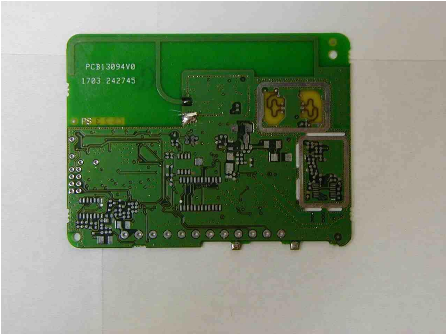
Figure 8 PCB Shields Removed
