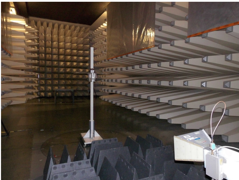
Setup for radiated emission
