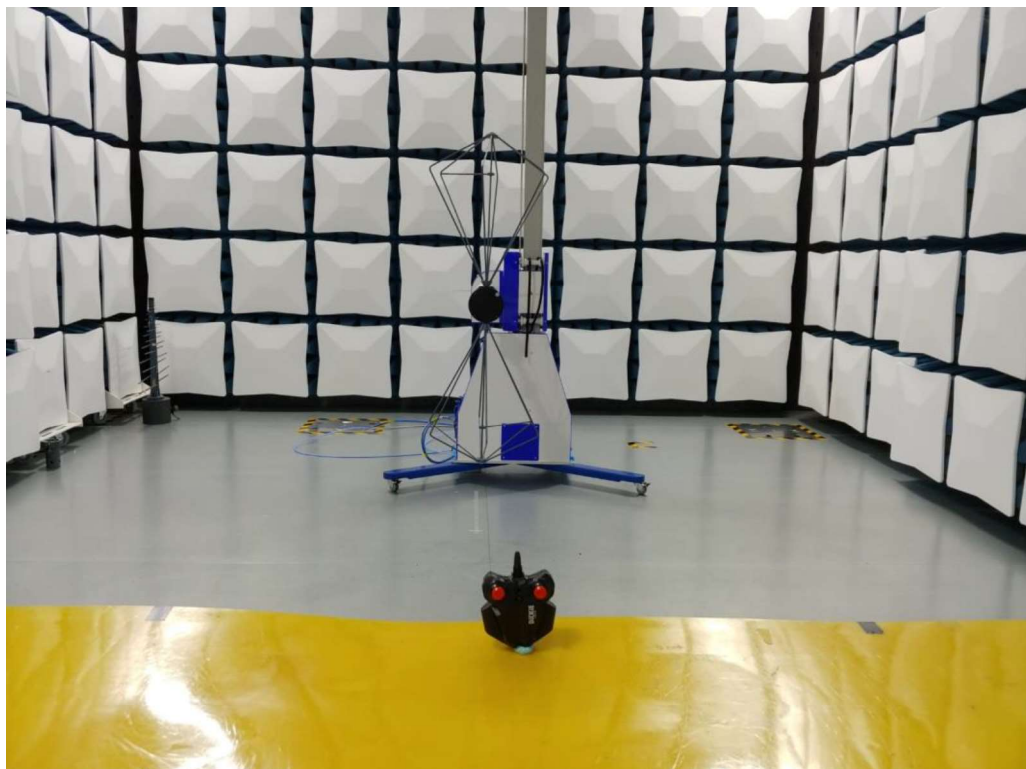
Set-up for Radiated Emission (30-200MHz)
