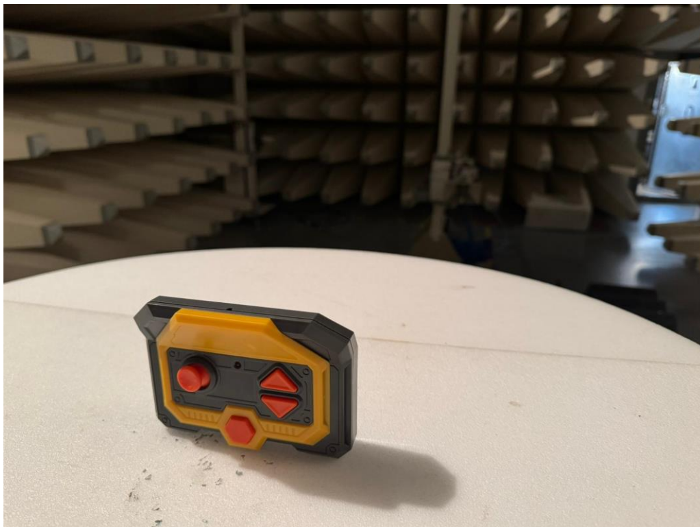
Set-up for Radiated Emission (1 GHz above)
