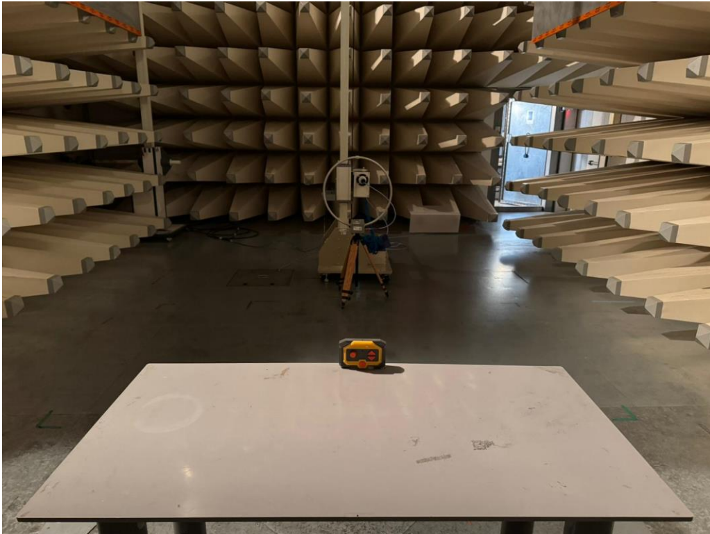
Set-up for Radiated Emission (9 kHz-30 MHz)
