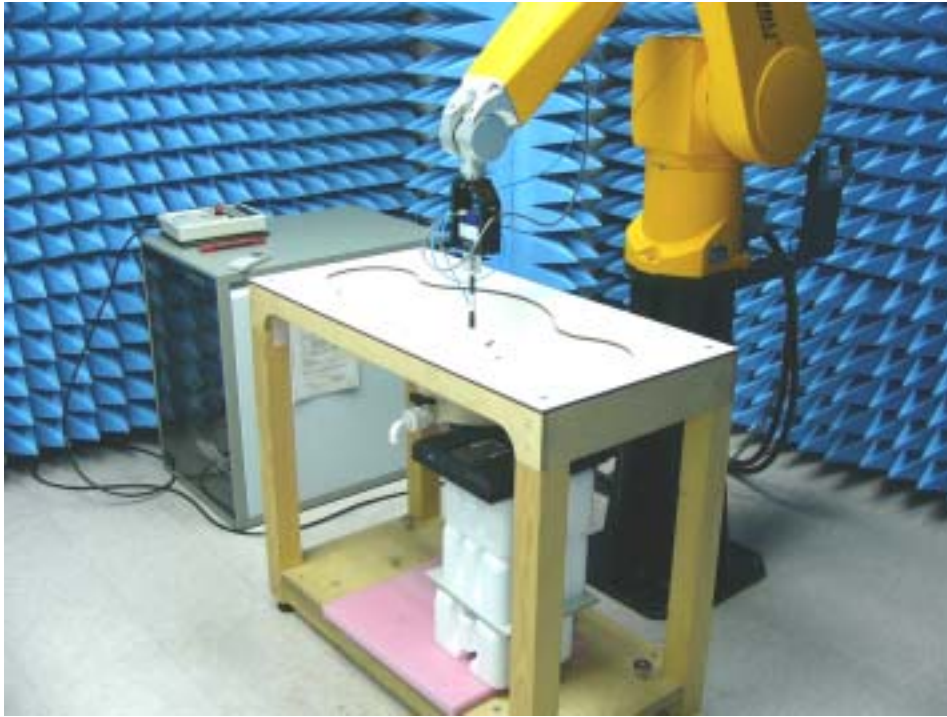
Fig.1 Photograph of the SAR measurement System
