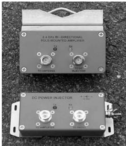
View showing the DC Injector and the pole mounted outdoor Amplifier attached to its mounting bracket.
