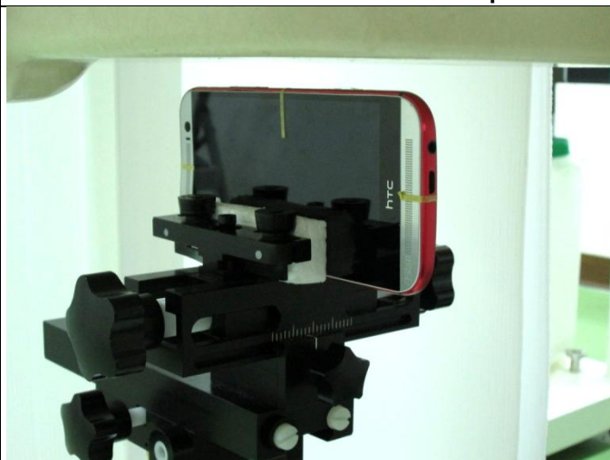
Right Side of EUT with 1.0 cm Gap
