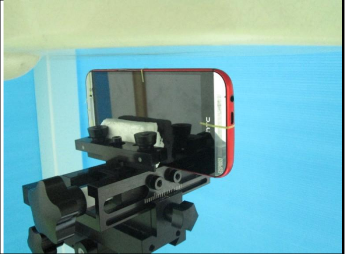
Right Side of EUT with 1.0 cm Gap
