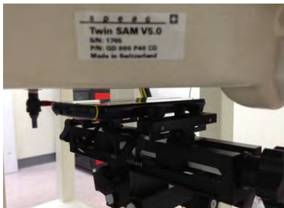
Fig.10 EUT front to flat phantom
