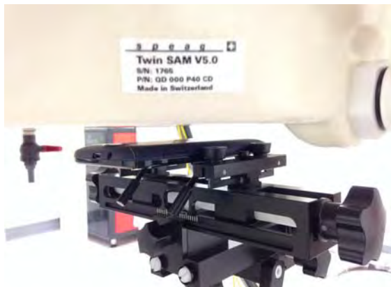
Fig.9 EUT back to flat phantom
