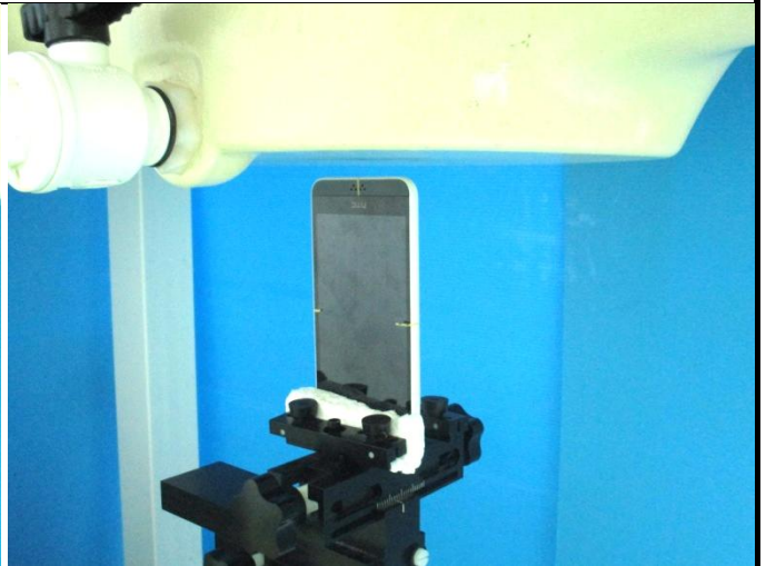
Bottom Side of EUT with 1.0 cm Gap
