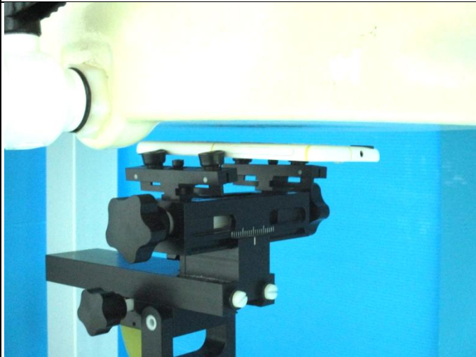
Rear Face of EUT with 1.0 cm Gap
