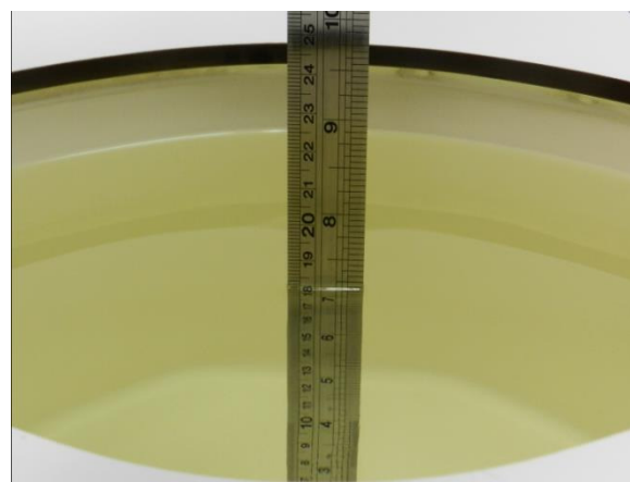
Fig 10.2 Photo of Liquid Height for Body SAR
