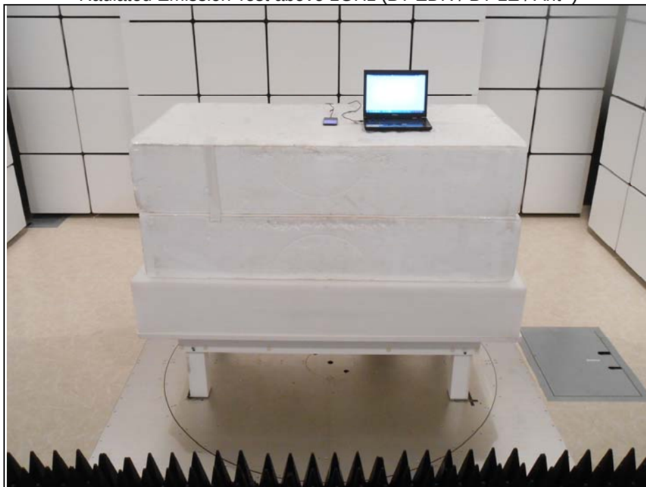
Radiated Emission Test above 1GHz (BT EDR / BT LE / Ant+)
