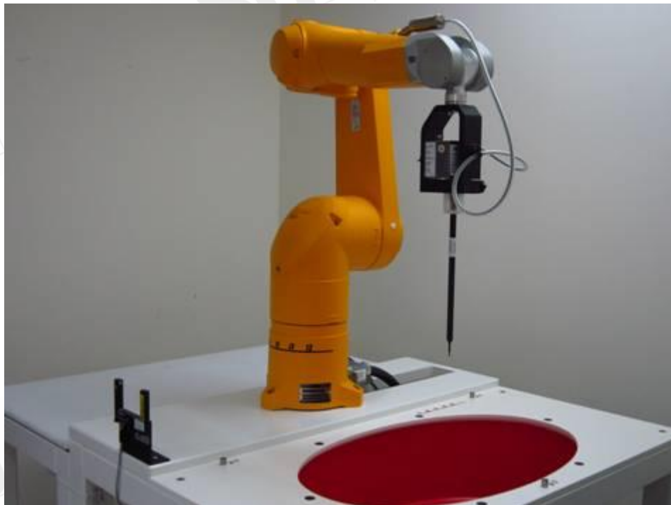
Fig.1 Photograph of the SAR measurement system
