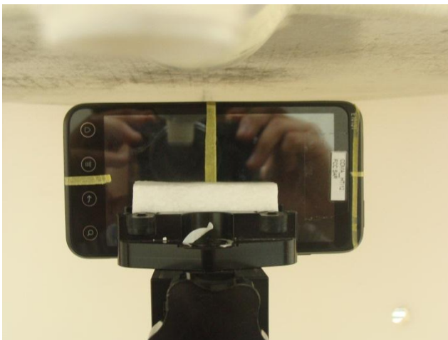
Left Side of the DUT with Phantom 0.5 cm Gap for DUT without Earphone
