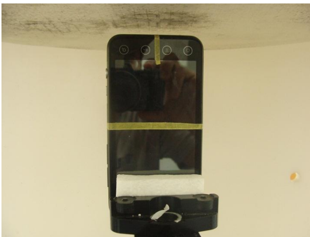
Bottom Side of the DUT with Phantom 1.0 cm Gap for DUT without Earphone
