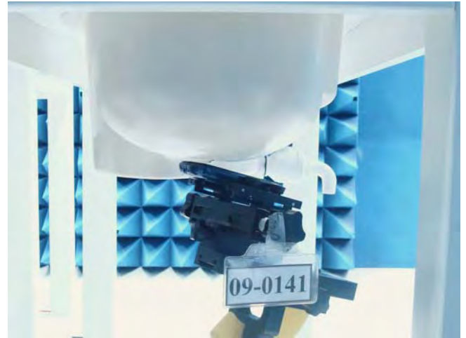
Figure 3. Right Head SAR Test Setup (Tilted)
