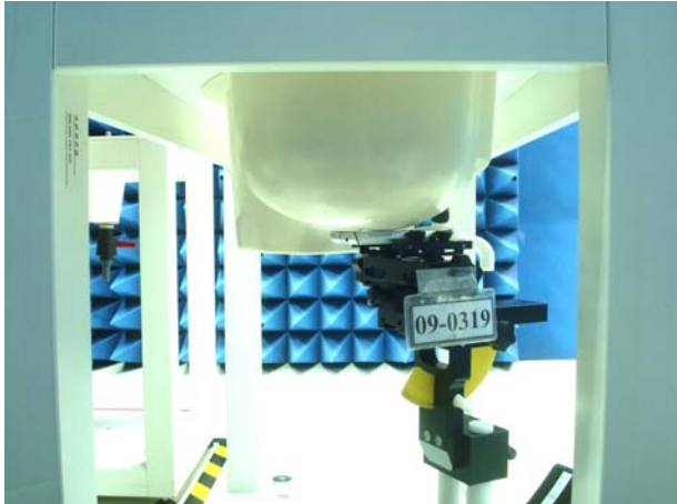
Figure 2. Right Head SAR Test Setup (Cheek)
