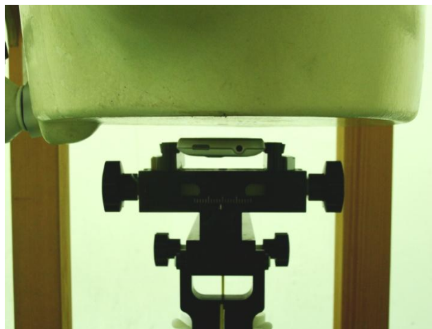
Front Face of the DUT with Phantom 1 cm Gap (DUT without Earphone)
